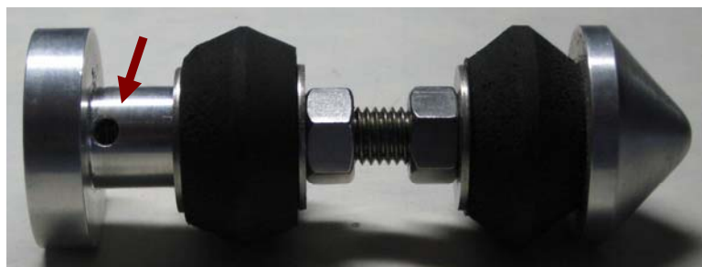
Figure 1. Livingstone piston with hole drilled through end plate.
